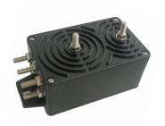
Voltage sensor using the principle of magnetic flux gate closed-loop can measure the voltage of various signals such as AC, DC, and mixed voltage under electrical isolation conditions. The high insulation between the primary and secondary edges ensures high accuracy, high linearity, long-term stability, and adaptability to various working environments.
