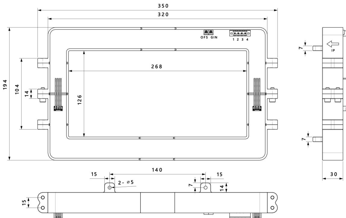
Elucidation: 1:+15V 2:-15V 3:V<sub>OUT</sub> 4:0V(GND) OFS:Zero adjustment GIN:Gain adjustment
